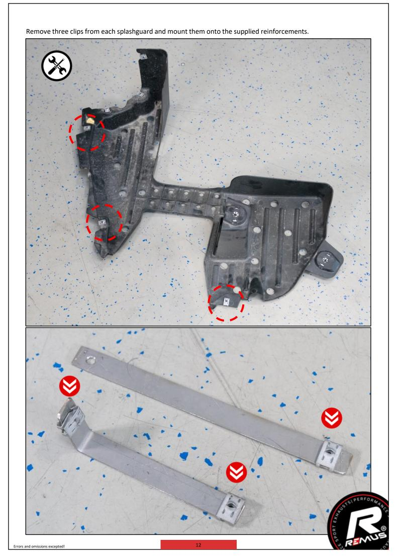
Mount the reinforcements on the left and right sides of the wheel arch cover/the rear bumper, use the stock bolds.
