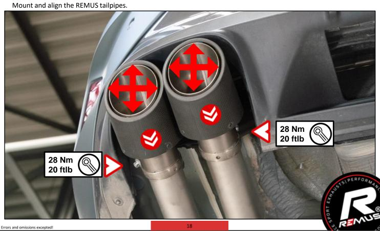
Align the exhaust system and tighten all connections.
