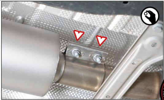
Install the REMUS connection tube onto the front silencer. Hang in the rubber.
