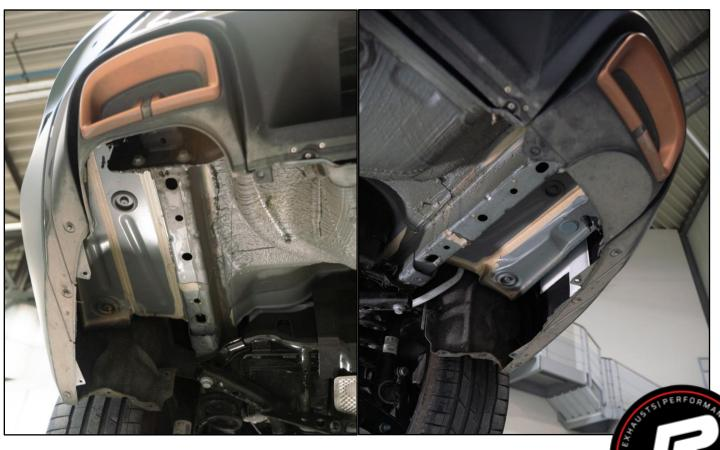
Remove the dummy tail pipe covers.
